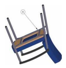
**A:** Turn the chair upside down and remove the upholstered seat cushion by removing the four #2 Philips wood screws.
