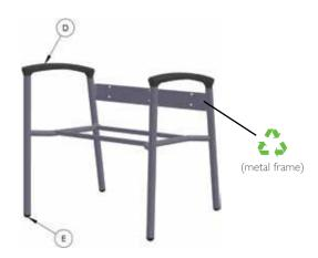
**D & E:** Place the chair on its side. Using firm blows with the hammer, knock the polyurethane arm free out of the frame. Next, take the flat blade screwdriver and hammer break the glides free from two of the legs. Flip the chair over and repeat the process for the other side.
